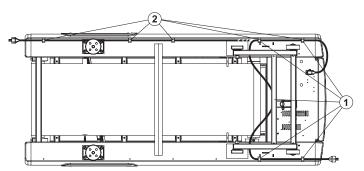
To plug the power cord into an outlet in front of the treadmill, use Hole Pattern 1 for outlets located at the front of the machine.
